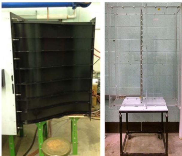
Fig. 5 A photo of the low turbulence (LT) 3.6 to 1 area contraction is shown on the left and a photo of the rectangular spool with the large grid (LG) is shown on the right
