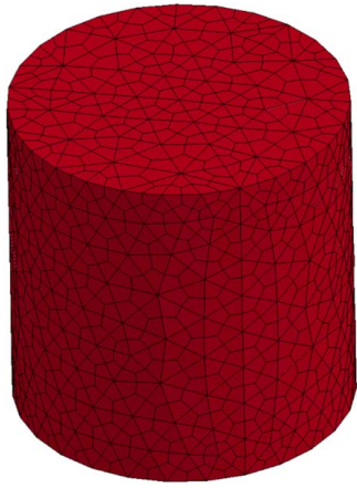
Fig. 3 A typical mesh of a cylindrical ice specimen ( D = 200 mm) for the MCNS model
