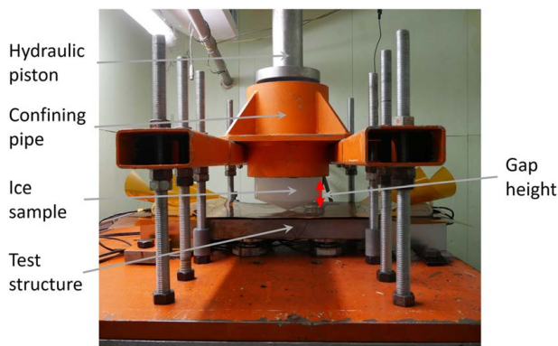
Fig. 8 Test setup of the ice extrusion test with a 200-mm ice specimen
