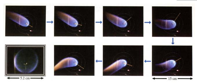
The Visualization of G-jitter Effects on a Burning Fuel Droplet in Reduced Gravity
