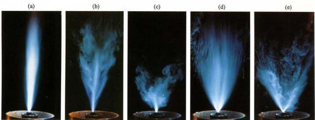
HEAT TRANSFER EFFECTS ON DROPLET VAPORIZATION BY AIR PREHEATING
