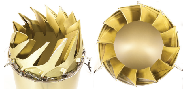
Fig. 4 Photographs of the assembled EAB nozzle: trimetric view (left) and aft-looking-forward view (right)
