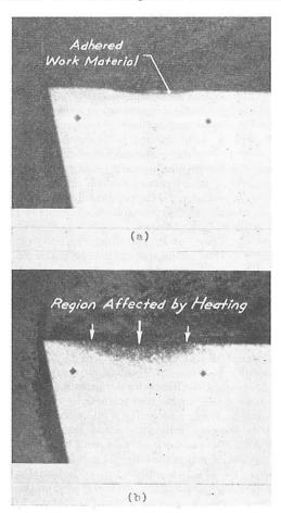
Feed:  $t_1 = 0.00979$  ipr Cutting time: 1.20 min
