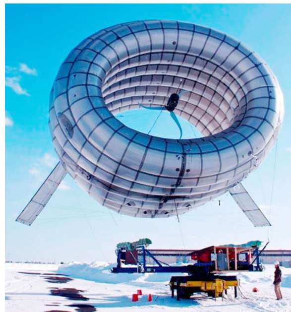
Fig. 2 Image of prototype full-scale system, the Altaeros BAT, showing annular shroud, turbine, tethers, and ground station (Adapted from Ref. [5])
