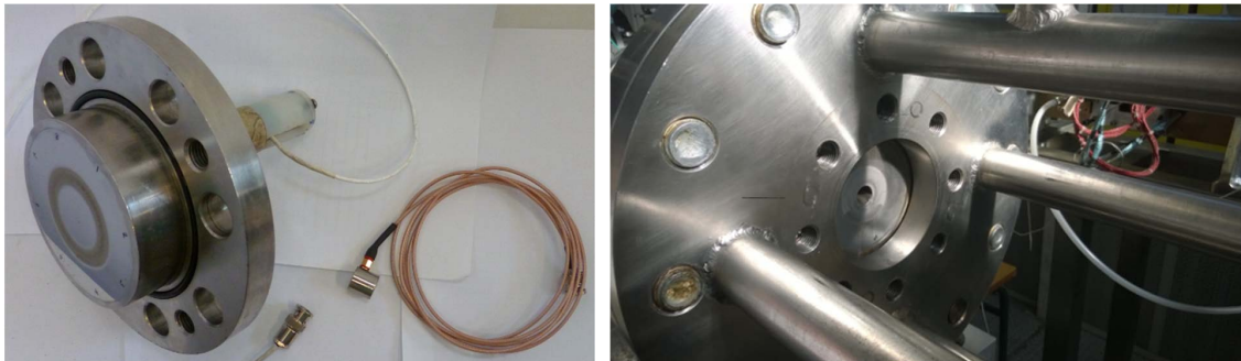
Figures 1(a) and 1(b). 1(a): Sample mounted to the sample holder and fitted with an AE sensor and a waveguide. 1(b): PREVERO test section opened and with the inlet nozzle in the middle. The sample is flush mounted so that it forms a part of the other wall in the test section.
