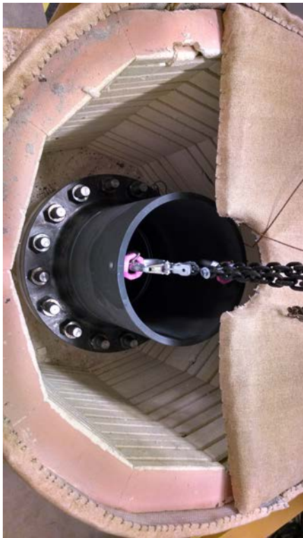
Figure 6: Assembly 1 suspended in the kiln before heating.
