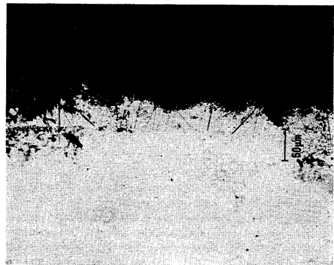
FIGURE 9: MORPHOLOGY OF HOT CORROSION OF PtAl ON MARM002DS AFTER 700 HR IN HOT RIG TEST. 200X, UNETCHED
