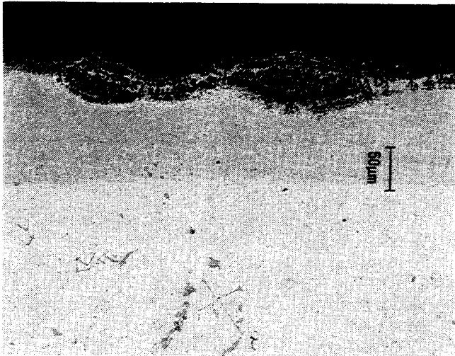
FIGURE 7: MORPHOLOGY OF HOT CORROSION OF SERMALOY 1515 SILICON-MODIFIED ALUMINIDE ON MARM002DS AFTER 750 HR IN HOT RIG TEST. 200X, UNETCHED
