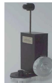
FIGURE 2: IMAGE OF AN EPISCLERAL VENOMANOMETER (EyeTech EV-310) THAT IS COMMERCIALY AVAILABLE [13].
