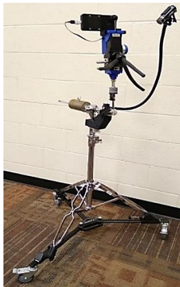
FIGURE 10: A COMPLETE ASSEMBLY OF THE PORTABLE VENOMANOMETER SYSTEM.
