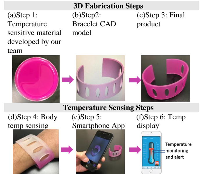
Figure 2: Temperature sensor development and operating demonstration: (a) the resin used to create the temperature sensor, (b) bracelet-shaped sensor model, (c) 3D-printed sensor, (d) demonstration of sensor changing color with body temperature, (e) and (f) smartphone app for temperature measurement and alerting.
