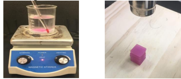
Figure 5: experimental setup for (a) activation temperature determination and (b) color change rate of the thermochromic material.
